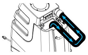
Connect a vacuum hose to the Cuff-Lynx<sup>™</sup> connection. Switch on the vacuum(s) and insert the vacuum hose into the solution tank to suck out all the unused solution. When finished, lift the recovery tank dump valve to drain.
