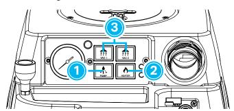
**1.** Turn pump switch on. Pull the lever on the cleaning tool to release air in the line. Hold lever until a steady flow of water comes out of the wand.
