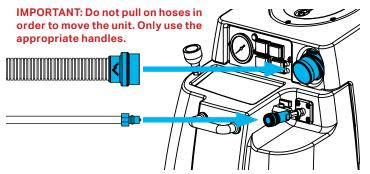
Use the included Cuff-Lynx<sup>™</sup> hose connectors to connect 1.5" or 2" vacuum hose to the Speedster<sup>®</sup>. Connect the solution hose via the quick connect fitting on the front of the Speedster<sup>®</sup>. ◆
