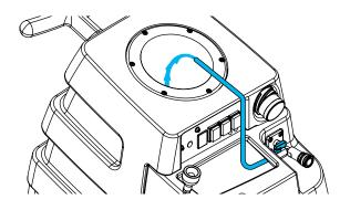
Rinse out the recovery tank using the wash hose inside the solution tank. Take the lid off the recovery tank and place the end of the wash hose inside. With solution or clean water in the solution tank, switch on the pump and turn the prime valve to position 1 (shown in section 2.5 on previous page). Rinse off the inside of the recovery tank and then drain the tank. •
