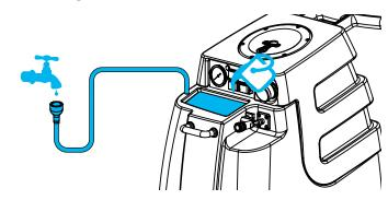
The Speedster<sup>®</sup> solution tank can be filled up via the faucet fill hose or from a bucket via the opening under the solution tank lid.
