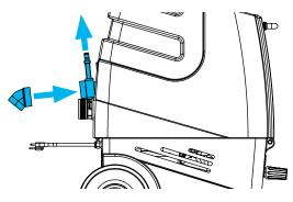
Empty the recovery tank by attaching the H226 45° drain elbow to the drain spout in back. Lift up the dump valve and empty the tank into a bucket or drain.
