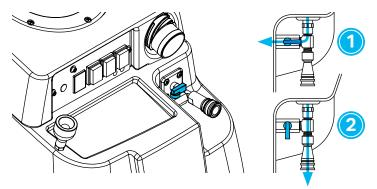
The Speedster® units come with a prime valve attached to the solution hose quick connect fitting. Turning the valve lever to position 1 directs flow towards the wash hose inside the solution tank. Turning the lever to position 2 directs flow towards the cleaning tool. ◆
